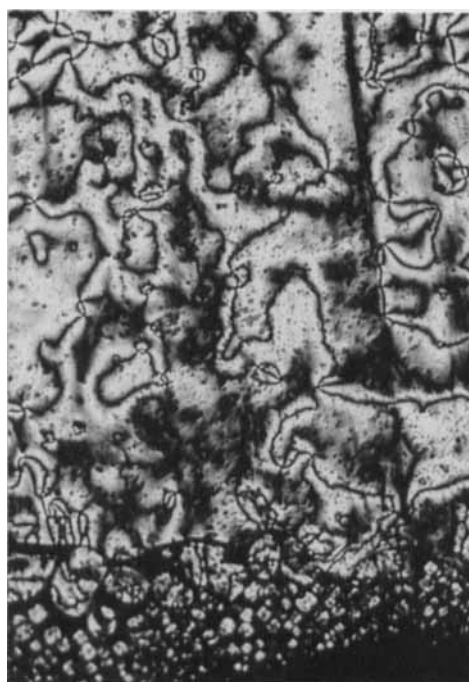
Figure 4. Polarizing light microscopic texture of the 4-hexyloxyphenyl 4-vinyl benzoate at 85°C.
